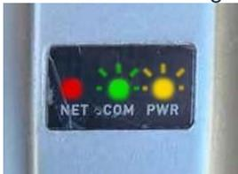
13: Once all LEDs are lit, briefly press the reset button on the Solis firmware update stick and the LEDs will flash very quickly at first and then more slowly.
