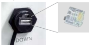
Plug in COM Resistor
